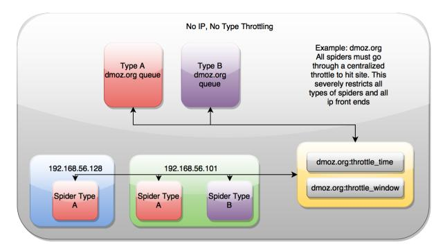
No throttle style dictates that the domain coordination is done through a single place. It is indifferent to the spider or the IP addresses of the machines crawling, ensuring they are all rate limited by one mechanism only.
