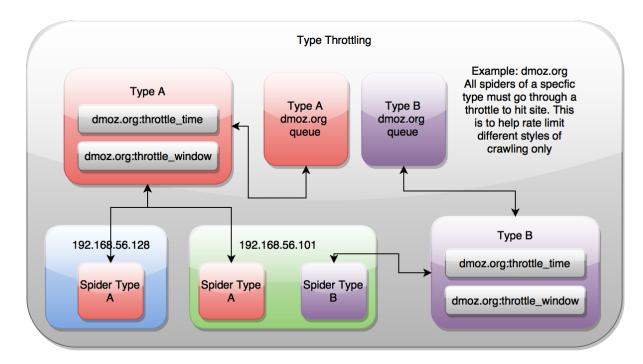
Type throttling means that for each domain, spiders of a different type (ie A, B, link, foo) will orchestrate with themselves to control how fast the cluster hits the domain. This disregards the public IP address of the machines that the Scrapy requests are routed through, so spiders on different machines are throttled based on how fast all of the other spiders in the cluster have hit that particular domain.
